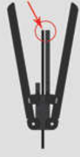
2. Insert the cable into the cable stripper, strip the cable as per the markings.
